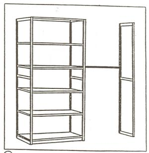
B ADD EXTRA SECTIONS BY USING KEY-HOLE SLOTS ON COMMON "T" UPRIGHTS. FOLLOW SAME SEQUENCE OF ASSEMBLY AS DETAILED IN PREVIOUS ILLUSTRATIONS.
